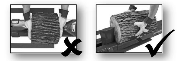
★ Hands should not be lower than half way down the sides of the block when splitting. If hands are lower and a log falls, fingers may get pinched between the log and the shelves.
