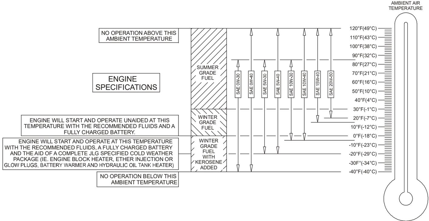
Figure 7-1. Engine Operating Temperature Specifications - Deutz - Sheet 1 of 2
