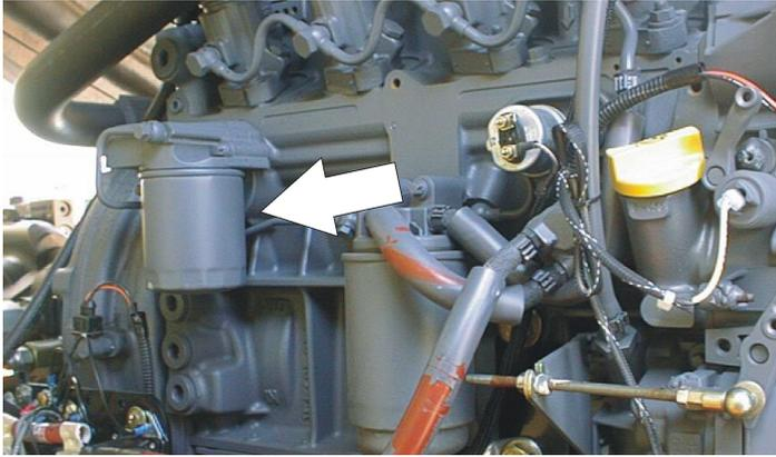
Lube Point(s) - Fill Cap/Spin-on Element
