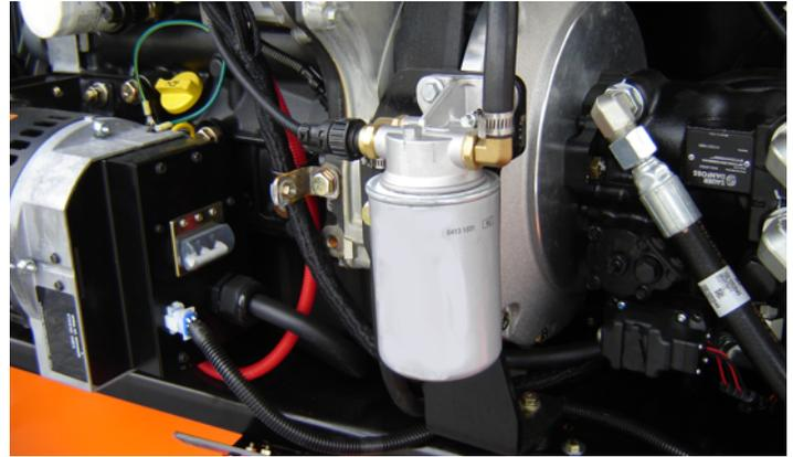
Lube Point(s) - Replaceable Element
