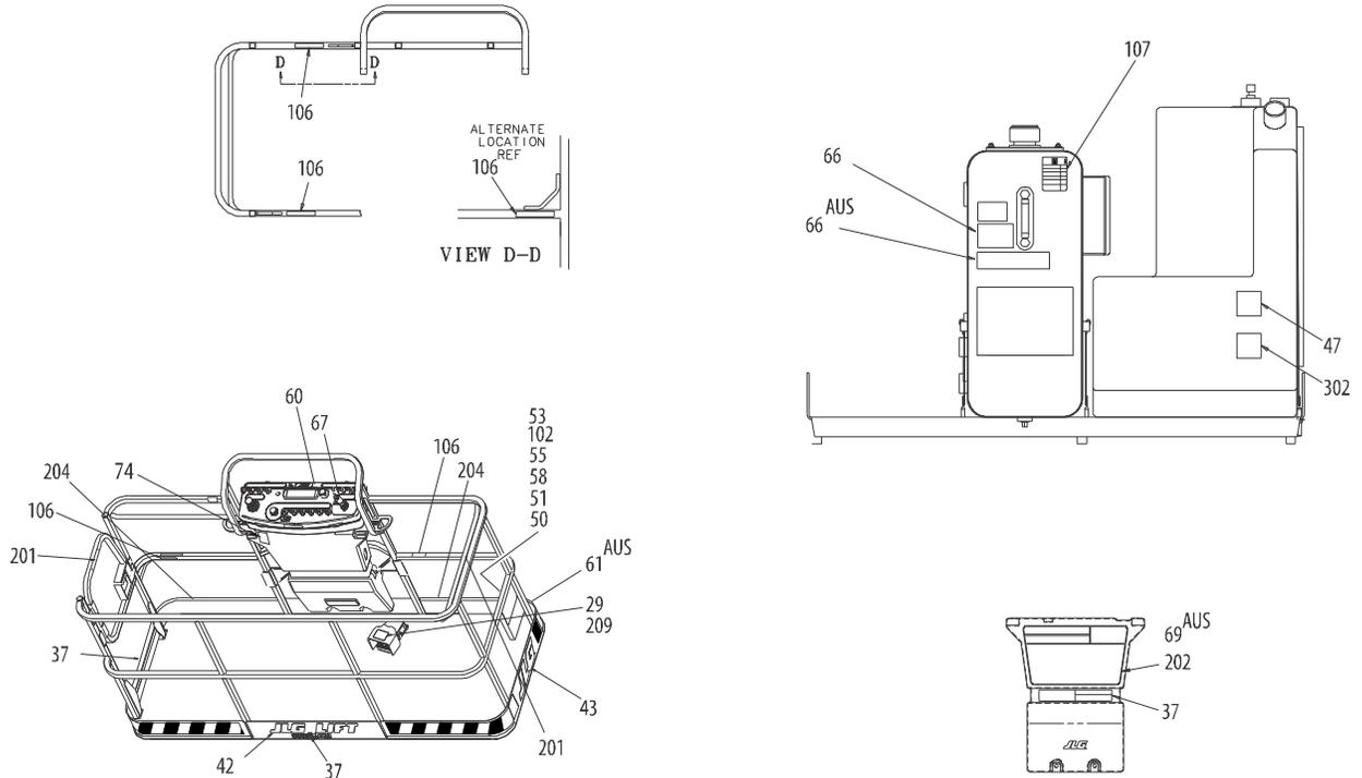
**Figure 4-10. 600AJ Decal Installation - Sheet 3 of 4**
