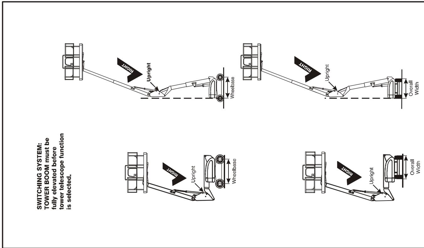
Figure 4-4. Boom Upright Positioning - Sheet 1 of 2
