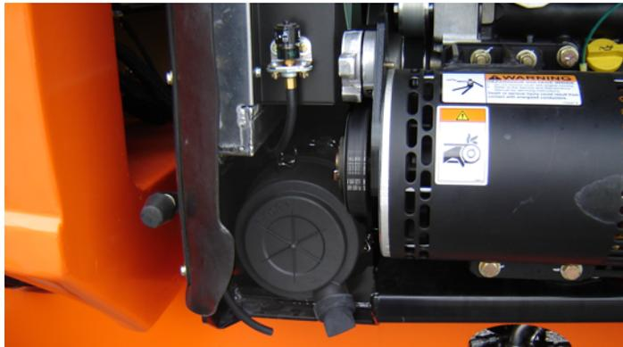
Lube Point(s) - Replaceable Element
