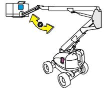
**NOTE:** When Power/Emergency Stop switch is in the "On" position and engine is not running, an alarm will sound, indicating Ignition is "On".
