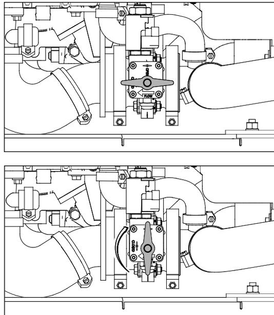
Figure 4-1. ASOV Reset (Closed to Open Position)
