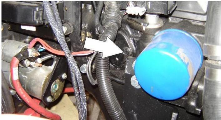
Lube Point(s) - Fill Cap/Spin-on Element
