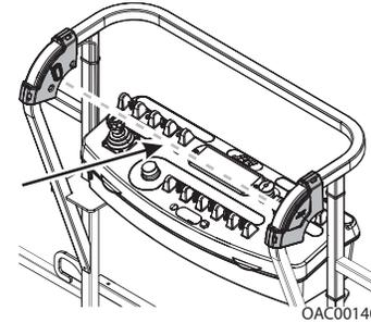
Operator passes through path of sensor beam.
