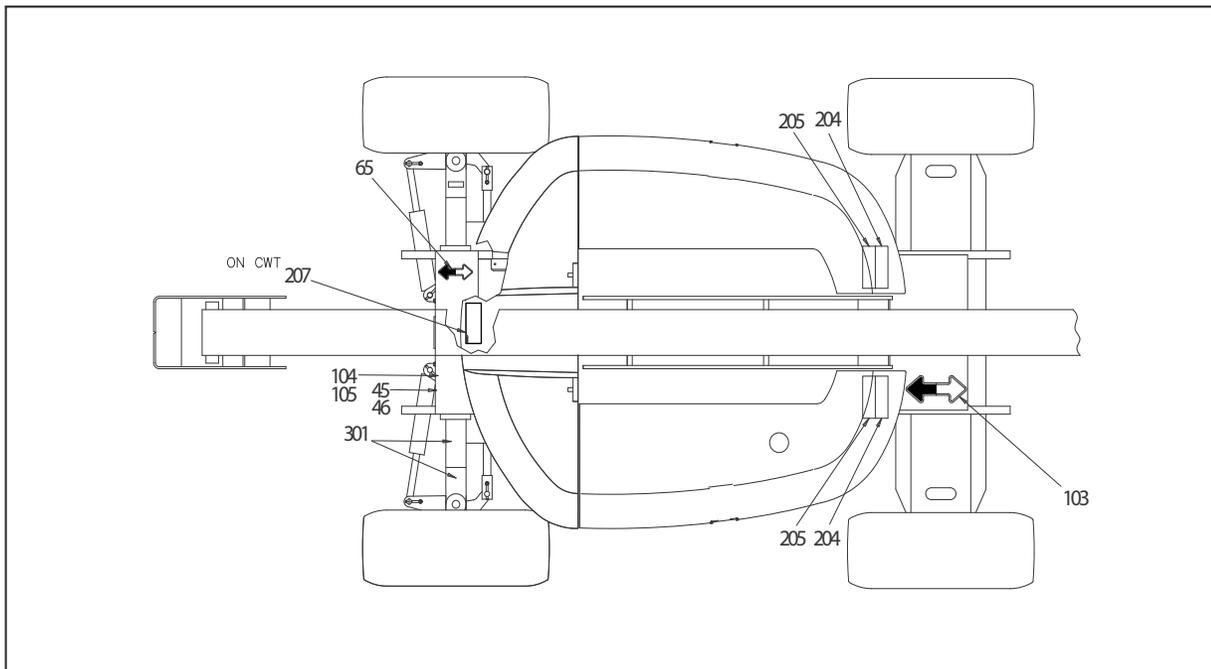
**Figure 4-11. 600AJ Decal Installation - Sheet 4 of 4**
