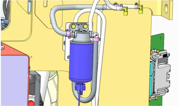
Lube Point(s) - Replaceable Element
