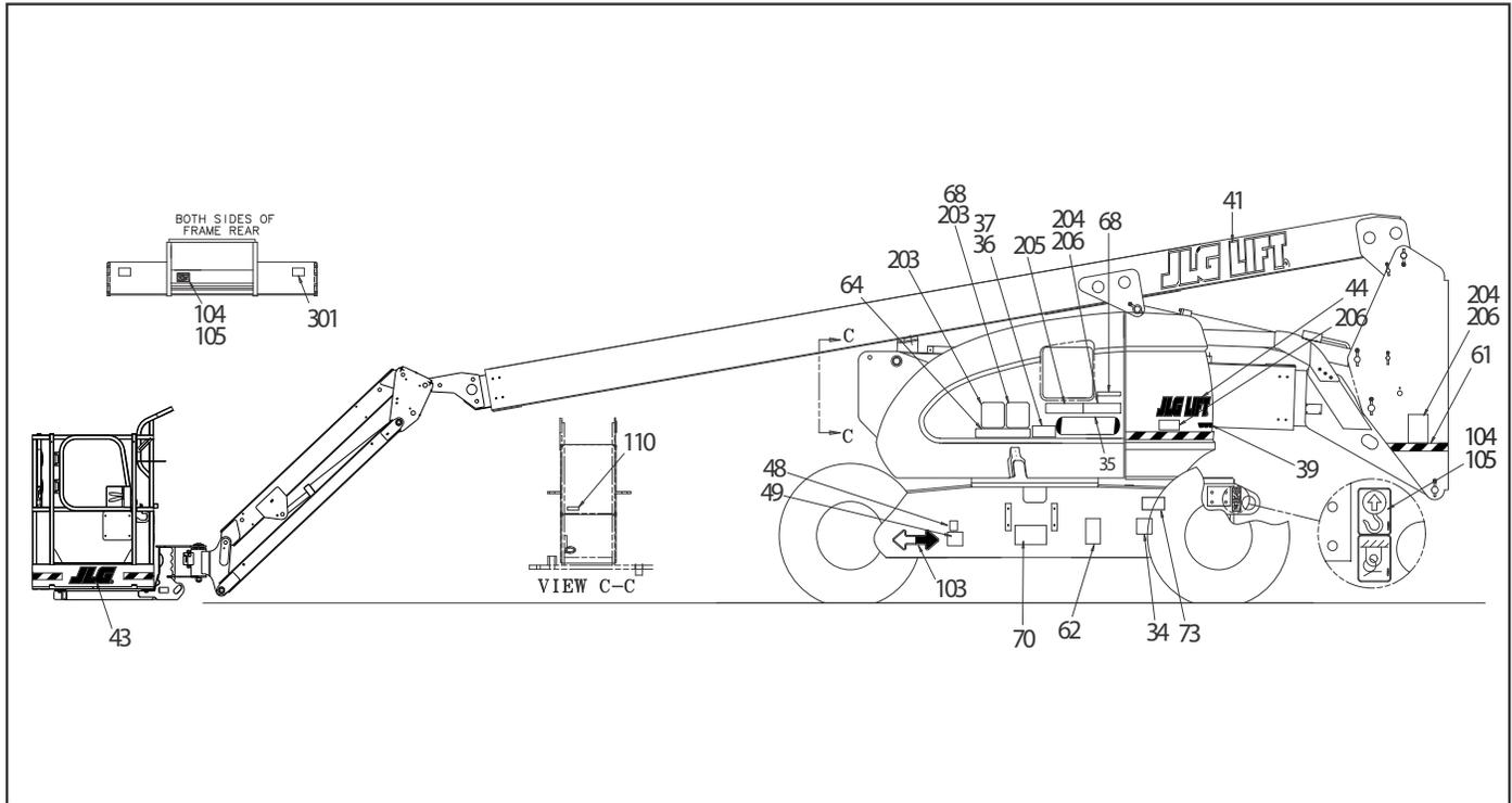
Figure 4-8. 600AJ Decal Installation - Sheet 1 of 4
