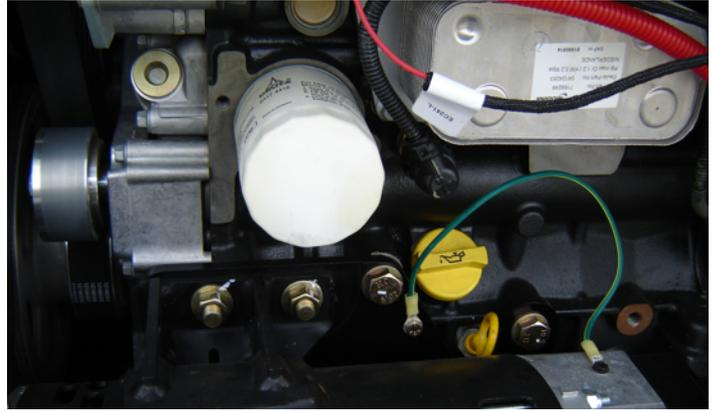
Lube Point(s) - Fill Cap/Spin-on Element
