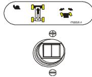
This machine is equipped with a Drive Orientation Indicator. The yellow light on the platform control console indicates that the boom is swung beyond the rear drive tires and the machine may Drive/Steer in the opposite direction from the movement of the controls. If the indicator is illuminated, operate the Drive function in the following manner:
