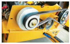
**THE CENTRIFUGAL CLUTCH** engagement prevents belt slip when engaging the clutch which means fewer maintenance costs.
