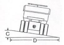
To calculate Grade, divide the vertical rise by the horizontal run and multiply by 100.
