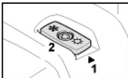
An arrow (Pos. 1) on the shroud indicates the setting of the shutter (Pos. 2) for summer or winter operation.
