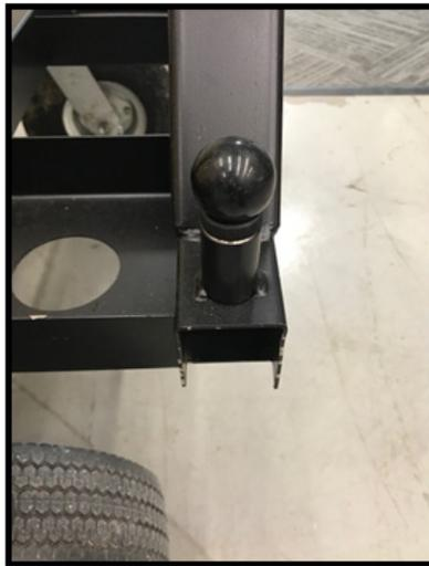
Spring pin and receiver for outriggers
