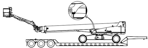
Note: Platform stowing for transport can only be done from the platform controls.
