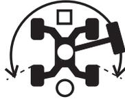
To drive, move the drive enable switch and slowly move the drive/steer control handle off center.
