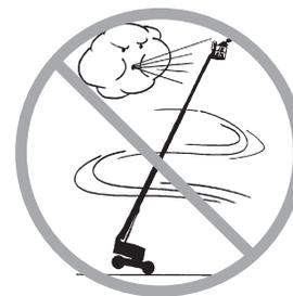
Do not raise the boom when wind speeds may exceed 28 mph / 12.5 m/s. If wind speeds exceed 28 mph / 12.5 m/s when the boom is raised, lower the boom and do not continue to operate the machine.
