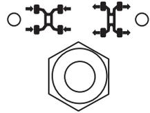
The axle extend and retract indicator lights will flash while the axles are moving. The axle extend indicator light will stay on when the axles are fully extended. The axle retract indicator light will stay on when the axles are fully retracted.
