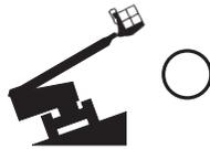
**Platform Not Level indicator light flashing:** The tilt alarm will be sounding when this light is flashing. The Platform Level toggle switch will only work in the direction that will level the platform. Level the platform until the indicator light is off.
