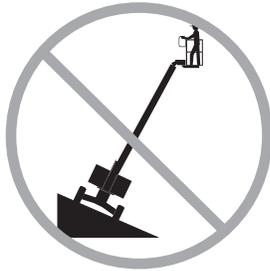
Do not raise or extend the boom unless the machine is on a firm, level surface.
