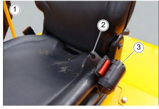
Figure 4.23 - Automatically Retracting Seat Belt
