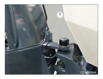
Figure 5.1 - Lifting Point
