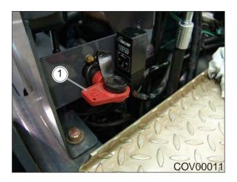
Figure 4.7 - Battery Isolator
