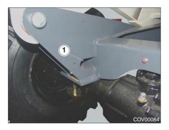
Figure 5.3. - Front Tie Down - Forward Tip Skip
