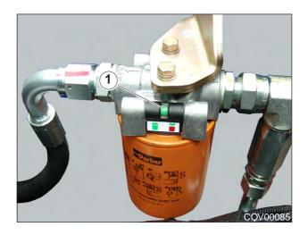
Figure 9.18 - Typical Hydraulic System Return Filter
