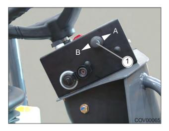
Figure 4.12 - Direction Indicator Switch
