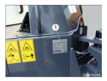
Figure 1.2 - Vehicle Identification Number Plate Location
