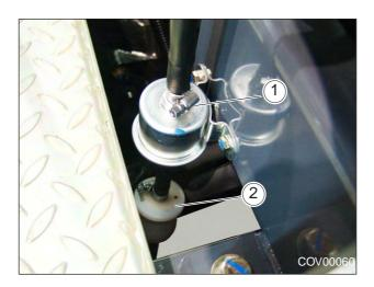
Figure 9.21 - In Line Fuel Filter
