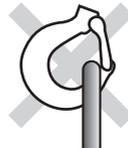
Suspended objects or slings are not hung in the proper position.
