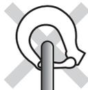
The tip of the hook is not capable of fully supporting the load.
