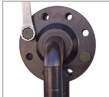
If necessary, use a second tool and turn until the bolt holes are in alignment and insert flange bolts.
