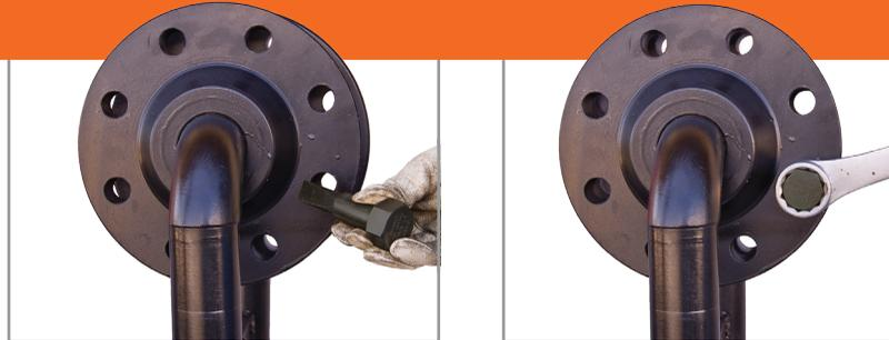
Find a bolt hole aligned enough for the tapered shaft to fit thru and turn.
